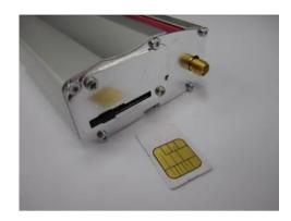
2. Slide the SIM card into the SIM holder.
