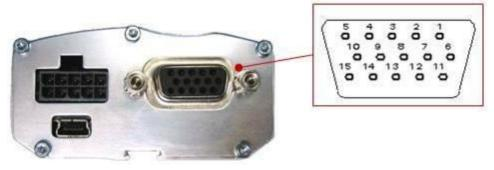
Figure 15. 15-Pin Serial Connector
