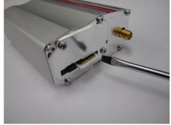
4. Slide the SIM lock switch to lock the SIM card in the Fastrack Xtend.
