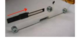
3. Connect the antenna to the main RF connector.
