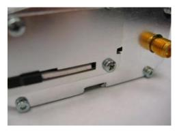
2. Slide the SIM lock switch to lock the SIM card in the Fastrack Xtend.
