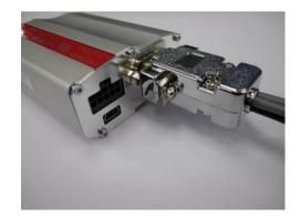
5. Plug the 6-wire cable accessory into the Fastrack Xtend and switch on the external power supply source.
