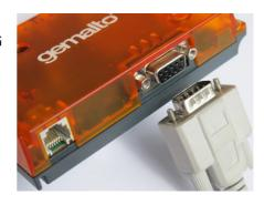
**4. Power Supply.** Plug the power supply DC output cable into the 3G Terminal and the mains cable with Fig-8 connector into the PSU and switch on.
