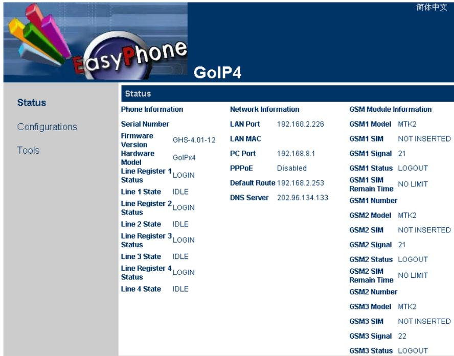
The image shows the 'GoIP4 Status' interface. It features a top header with the 'EasyPhone GoIP4' logo and a '简体中文' (Simplified Chinese) language selector. On the left, there is a navigation menu with 'Status', 'Configurations', and 'Tools'. The main content area is a table with the following structure:
