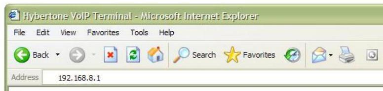
Open the Internet Explorer and enter 192.168.8.1 or <http://192.168.8.1> in the address bar, then, the login page is popped up for password input. Enter the login account ("admin" as default) in the User Name, and password ("admin" as default) in the Password field.
