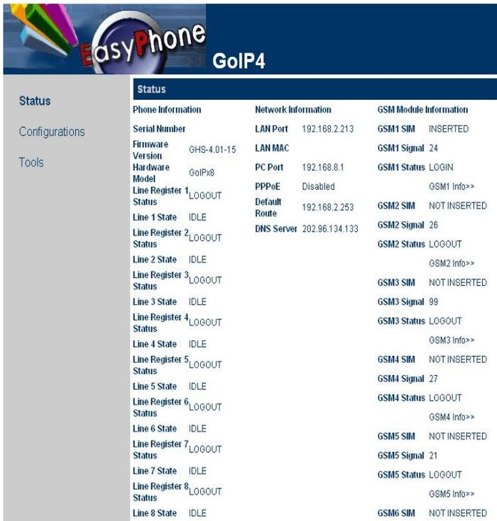
The image shows the 'GoIP8 Status' interface. It features a top header with the 'EasyPhone GoIP4' logo and a '简体中文' (Simplified Chinese) language selector. On the left, there is a navigation menu with 'Status', 'Configurations', and 'Tools'. The main content area is a table with the following structure:
