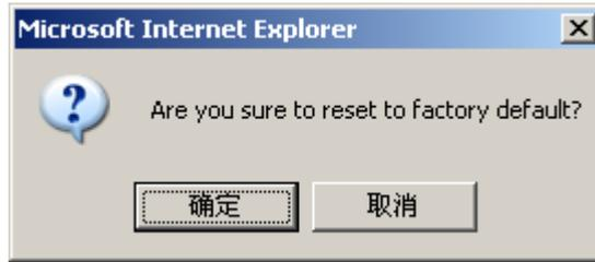
Click OK. All the parameters of the gateway will be cleared and the gateway will automatically restart. After the gateway is restarted, all the settings restore to the factory default settings. This feature can be completed by using the asterisk command. For details about this operation, see the section of “Asterisk Instructions”.
